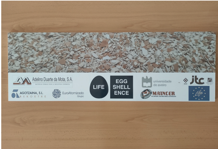
30x90 cm tiles glazed and fired at industrial scale.
